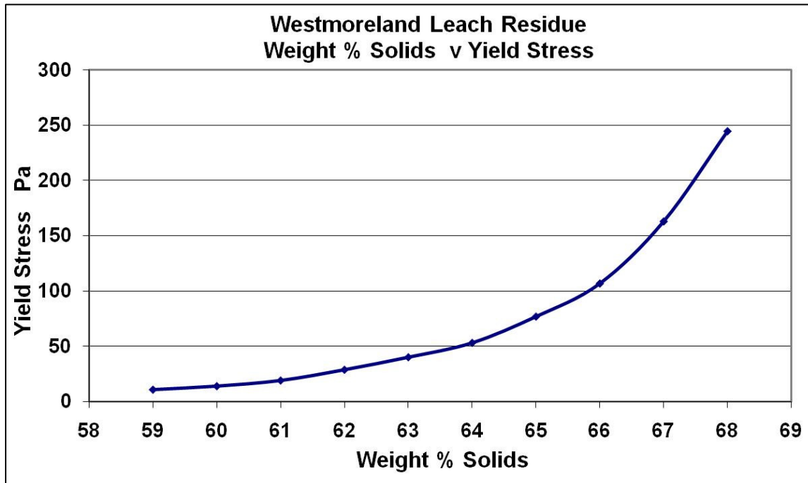
Figure 13.7 Thickened Pulp Yield Stress vs Slurry Solids Density – Bulk Sample
