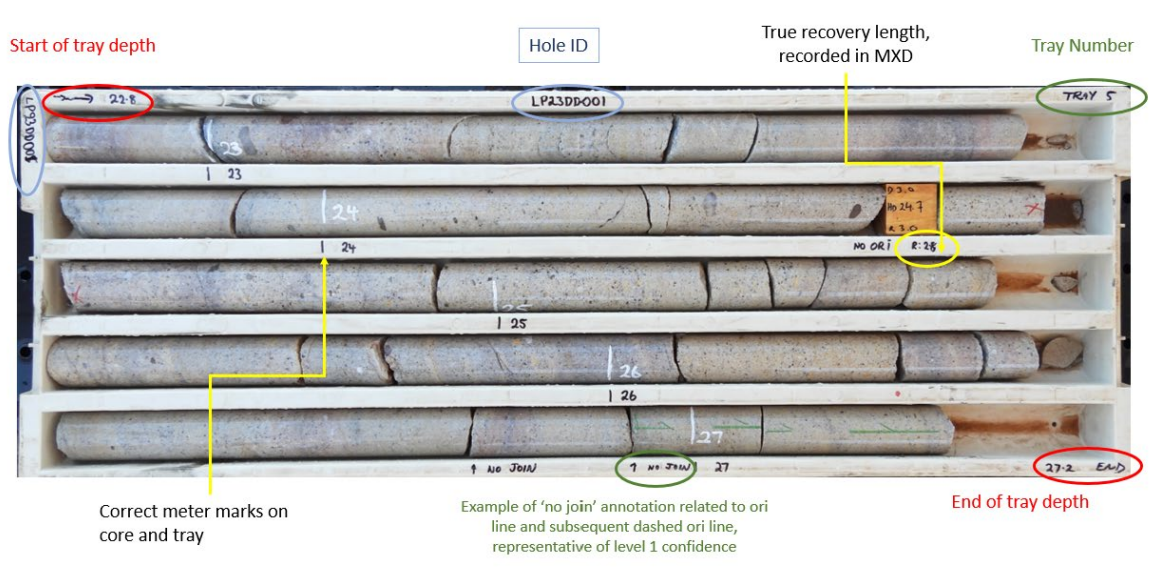
Figure 10.18 Example drill core marked up for cutting and sampling
